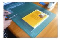
**STEP 1.** Pull film from roll, lay book face up on it leaving about 50mm on the top, right edge, and bottom. Turn the book and film to the left (same as picture). Cut film from the roll.
